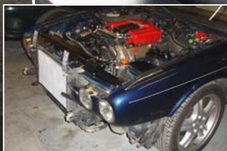
XK/XKR, S-TYPEs and X350 XJRs out there, and a lot get totalled!" To make the installation as easy as possible, though, the engine Danny was after was the 4.2-litre supercharged lump from a late X100 XKR. "Installing a previous generation XKR 4.2-litre engine is relatively straightforward, but with an S-TYPE R or X350 XJR unit there's an awful lot that has to be changed in terms of ancillaries."
