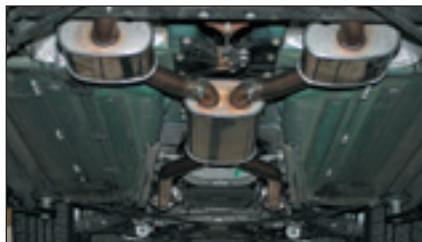
*The centre silencers have a balance pipe built in, this eliminates any possibility of horrible noises from back-draft emitting from the pipes on the over-run.*
