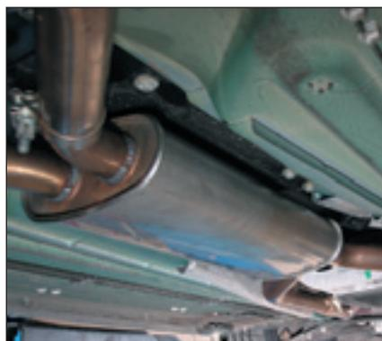
*The intermediate silencer can also be removed and replaced with straight pipes for those who want to increase performance and overall noise levels. Someone can buy the whole system and because of the use of olive joints over the rear axle pipes, the silencers can easily be removed, replaced with straight pipes for that "fun run", track day or for the whole summer but if going on an overseas journey, or for the winter, you can easily refit the silencer.*
