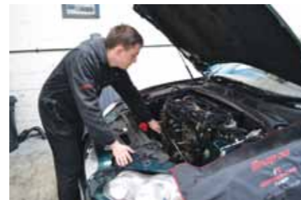
Technician Joe Horsley mid way through a full timing belt change on an XF 2.7 diesel
