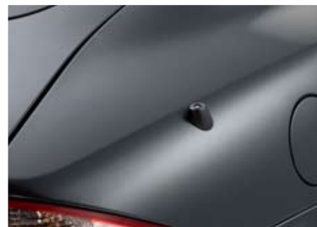
The XK pictured features the popular 20in Senta alloys – originally optional on both XKs and XKR, they became standard fitment to XKR with the 2008MY, and to the XK with the introduction of the XK60 model. For 2008MY cars on, the external antennae (below right) was replaced by an integrated spoiler/aerial unit
