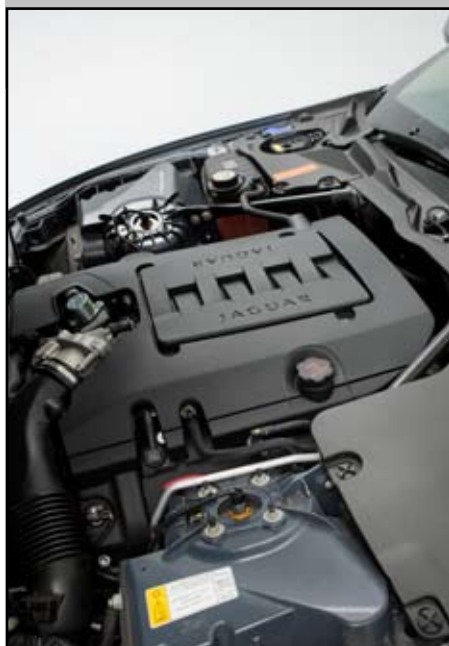
The view under the bonnet is not that exciting, but the 4.2-litre V8 is a reliable performer – note the cable from the strut top indicating that CATS is fitted
